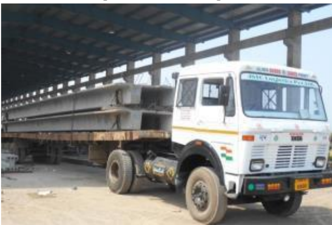
Single Tee Slab – Logistics
